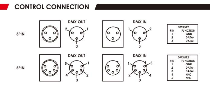
Connection between controller and projector and between one projector and another must be made with a 2 core-screened cable, with each core having at least a 0.5mm diameter. Connection to and from the projector is via cannon 3 pin (which are included with the projector) XLR plugs and sockets. The XLR's are connected as shown in the figure above.
