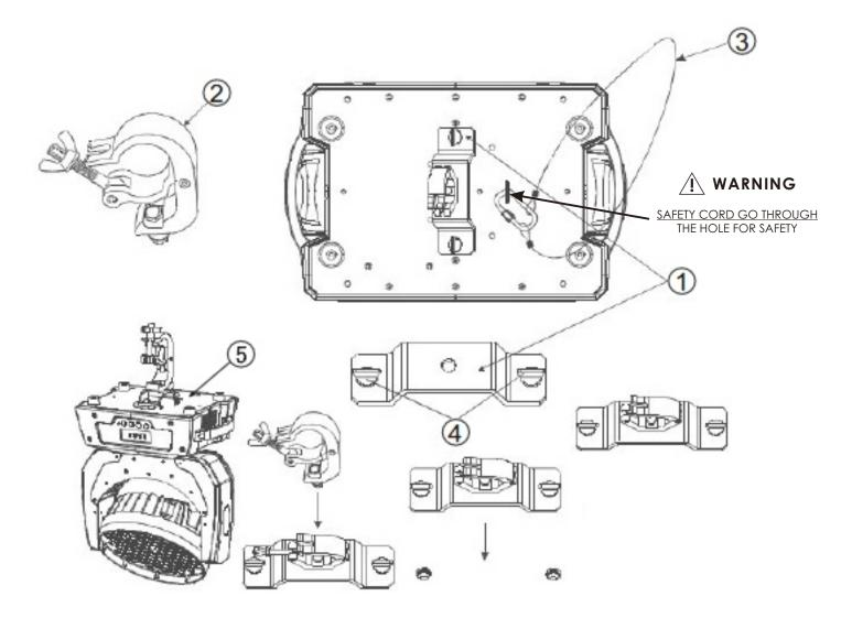
Take 1 clamp and 1 safety cord (the clamp and safety cord are optional accessories). Hang the fixture on the structure and fasten the screws attached to the clamp. (See the **WARNING** on the underside of the base as shown above) Always ensure that the projector is firmly anchored to avoid vibration and slipping whilst functioning. Always ensure that the structure that you are going to mount the projector is secure and is strong enough to support a weight of each projector.
