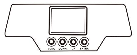
Projector configuration can be set conveniently via press button switch and LCD display. To browse or change its setup options, Press button <u>ENTER</u> to unlock panel. Menu will be displayed on the screen, each menu has it own sub-menu. Each menu has specific function, Please refer to "**Operation Menu**" for details.
